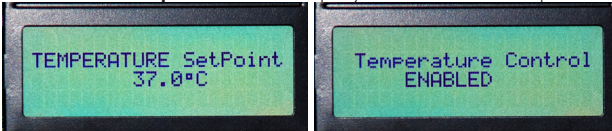
Fig. 8—(Left) The temperature display shows the current temperature setpoint.
