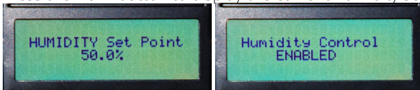
Fig. 13—(Left) The humidity display shows the current humidity setpoint.
