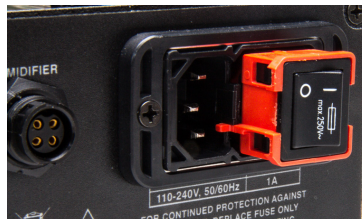
Fig. 27—(Left) Insert the screw driver under the fuse housing lip and pry the housing open.
