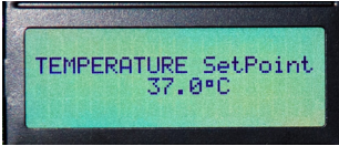
Fig. 6—Press TEMP to display the temperature setpoint.
